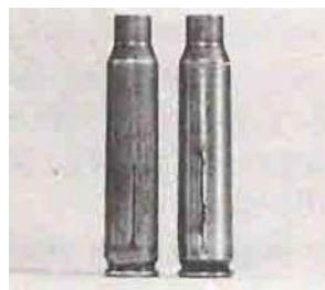
Figure 2: Centerfire case failures caused by manufacturing faults [7]
