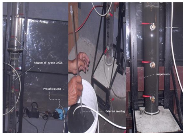
Figure 2. Process of external seeding to seeding and acclimatization process in huasb reactor
