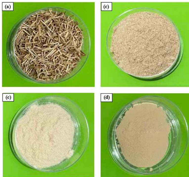
Figure 1. OPFF chopped (a), Raw OPFF (b), OPFF after chemical treatment (c), OPFF after mechanical treatment (d).
