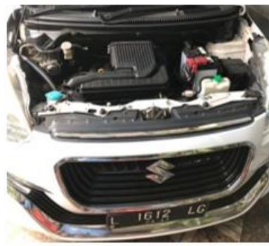
Figure 2. All New Ertiga Engine Model K14B DOHC-VVT 4 Cylinder 16 Valve Engine capacity 1.373 cc Maximum Power 95 Ps / 6.000 rpm Maximum Torque 130 Nm / 4.000 rpm
