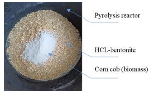
Fig. 2 position materials before pyrolysis process
