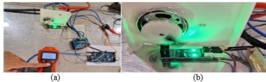
Figure 7. a. Measurement using a tachometer b. measurements using LM393
